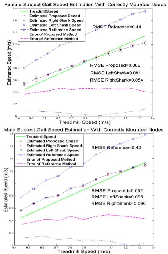
Figure 9. Gait speed estimation with correctly mounted nodes.
