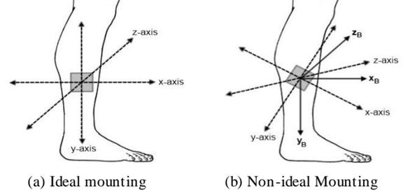
Figure 3. Coordinate in Body Frame, x-axis is defined as the walking direction, y-axis is the direction of gravity, z-axis is pointing inward. The dotted axes represent the basis vectors for the inertial frame, and the solid vectors represent the basis vectors for the global frame.
