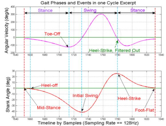
Figure 6. Comparison of angular velocity and shank angle in one gait cycle (counter-clockwise swing as positive in angular velocity).
