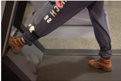
Figure 8. TEMPO nodes mounted nonideally out of sagittal plane.
