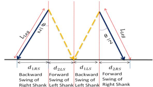
Figure 2. Reference Model [7], where  $L_{Leg}$  is the length of the leg,  $\theta$  is the shank angle range of one gait cycle measured in degrees.
