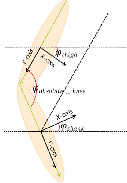
**Figure 2. Accelerometer placement and Knee joint angle.**
