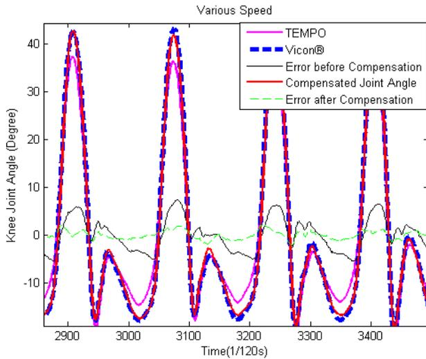
Figure 5 Cyclic Error Compensation Method
