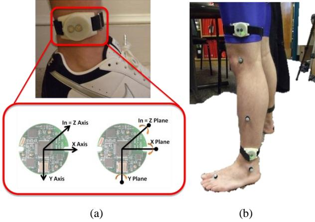
**Figure 1. (a) The TEMPO 3.1 node with mounting position, the TEMPO nodes are placed with the cephalic direction as Y-axis positive, the anterior direction as X-axis positive, and lateral direction as Z-axis positive. (b) The TEMPO nodes mounted on-body.**
